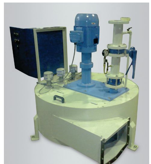
TANQUE REBOMBAMENTO COM CALHA PUMPING TANK WITH TROUGH
